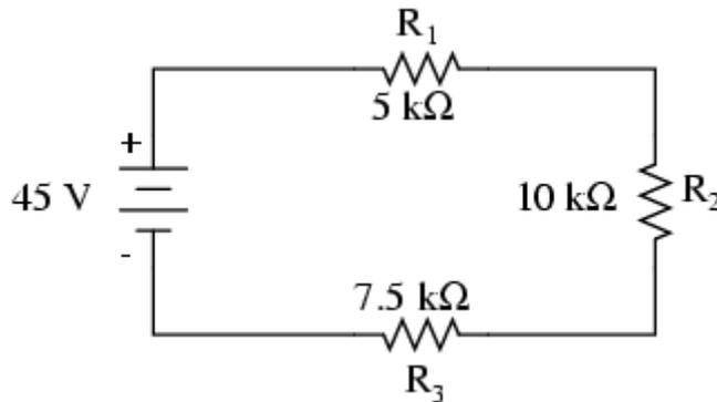
$$E_{R1} = 45 \text{ V} \frac{5 \text{ k}\Omega}{22.5 \text{ k}\Omega} = 10 \text{ V}$$
