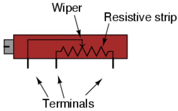
*Using a potentiometer as a variable voltage divider*
