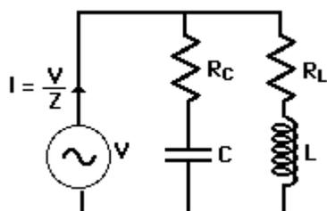
$$Z_{\text{equiv}} = \frac{Z_L Z_C}{Z_L + Z_C} = \frac{(R_L + j\omega L)(R_C - \frac{j}{\omega C})}{(R_L + R_C) + j(\omega L - \frac{1}{\omega C})}$$
