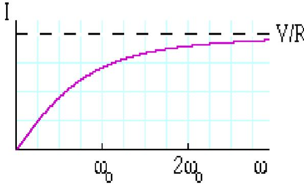
$$I = \frac{V_{source}}{\sqrt{R^2 + \left(\frac{1}{\omega C}\right)^2}}$$
